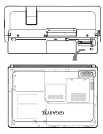
Line up the notebook with the docking station as shown above and make sure of the positioning. Once aligned gently place the notebook onto the docking station and press down firmly once aligned until the notebook is connected, you will hear a solid click to confirm that the notebook is then connected. The Battery light should come on to indicate that it is seated and connected properly. Ensure that the AC adaptor is connected first before connecting the notebook to the docking station.
